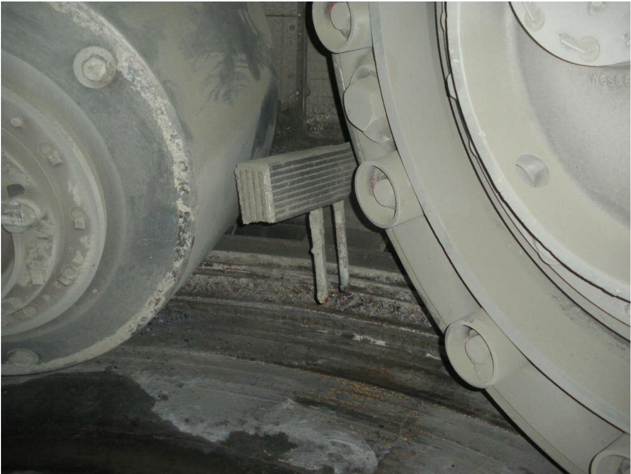
Figure 2 - By utilizing the water pipeline, the grinding aid enters the mill directly under the roller presses
