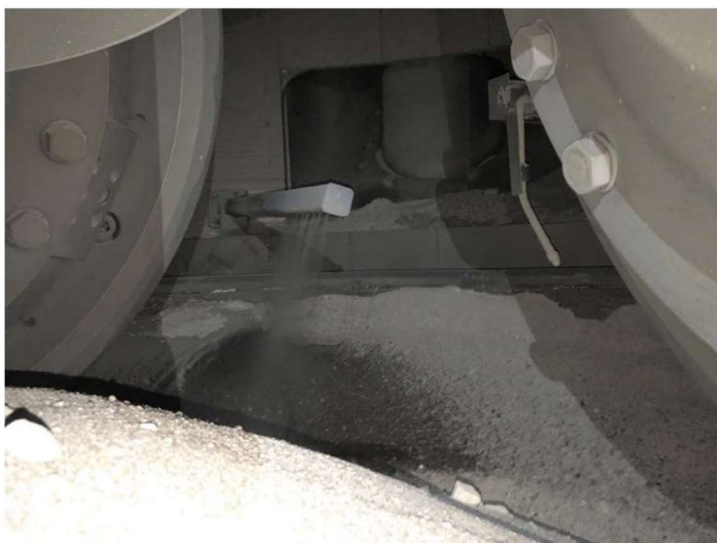
Figure 3. Spraying of cement additive on the grinding bed, close to roller.
