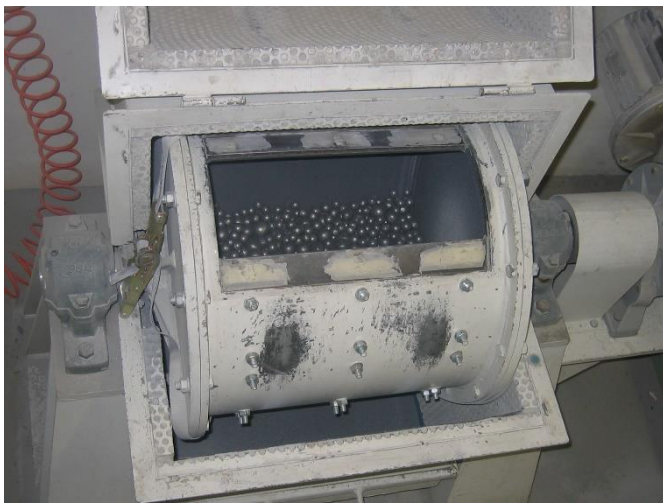
Figure 1: Laboratory ball mill for the reproduction of cements.
