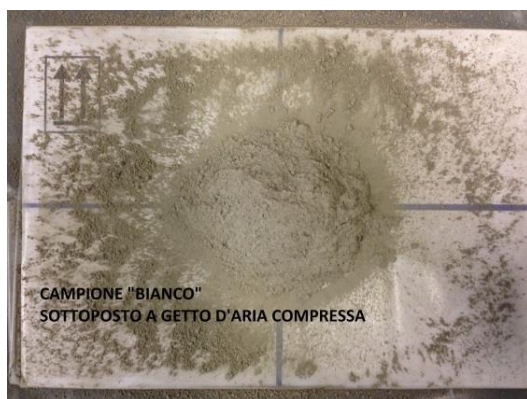
Image 1: blank sample – after compressed air jet
