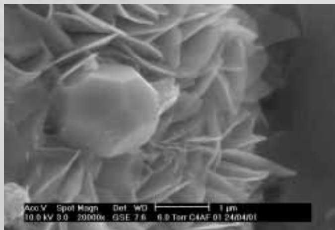
Figure 8 - ESEM-FEG image of synthetic C_4AF paste ( water/C_4AF = 0.4 ).
